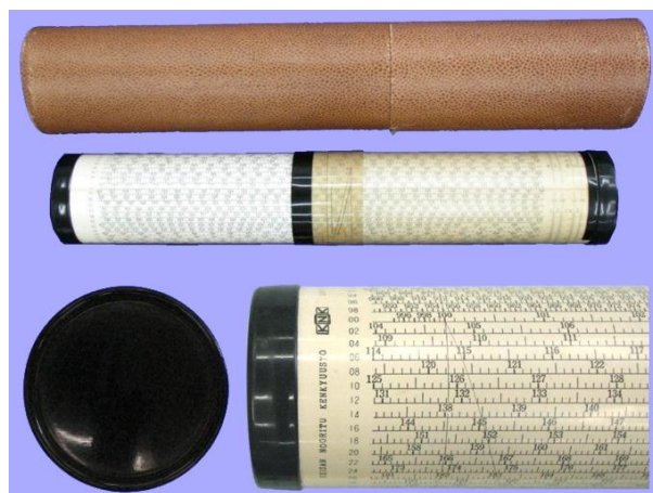
Fig.2 George Fuller type Slide rule (Preservation No.12011)
