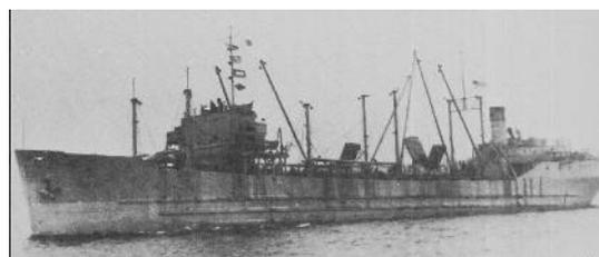
Fig. 5 C1SD1 type Concrete Cargo Ship
