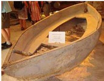
Fig. 1 First Concrete Boat
