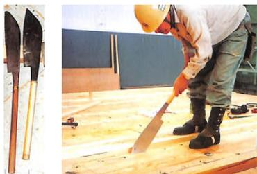
Fig.10 'Surinoko' saws for preparing the surface of plates to mate each other to keep water tightness
