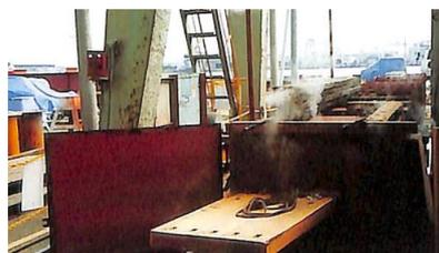
Fig. 9 Steam box for bending shell plates
