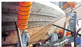
Fig.11 Forward shell structure called 'Yotoori'
