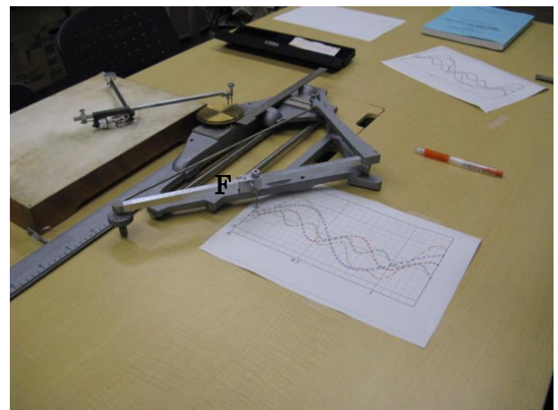
Fig. 7 Photo of calculating Fourier coefficients of a given test function, Eqn.10, by the Harmonic Analyzer .
