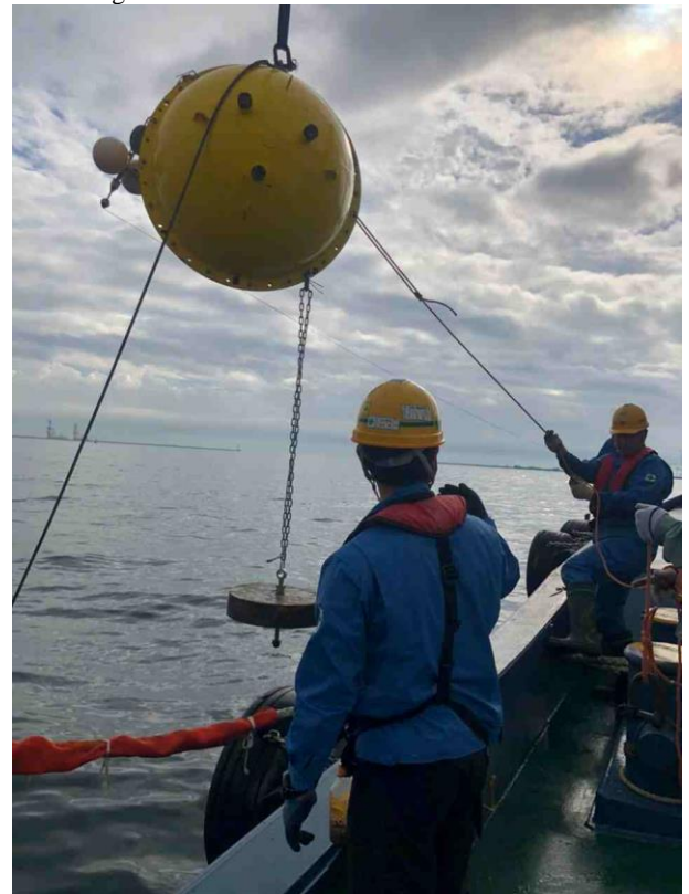
Fig. 11 Submersion test at Kobe port.
