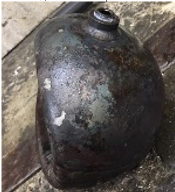
(c) Model collapsed by buckling
