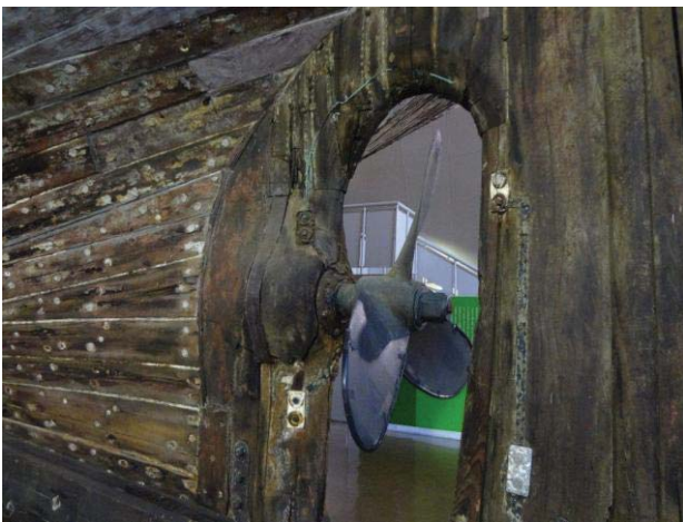
Fig.8 Propeller Aperture of Fukuryumaru No.5
