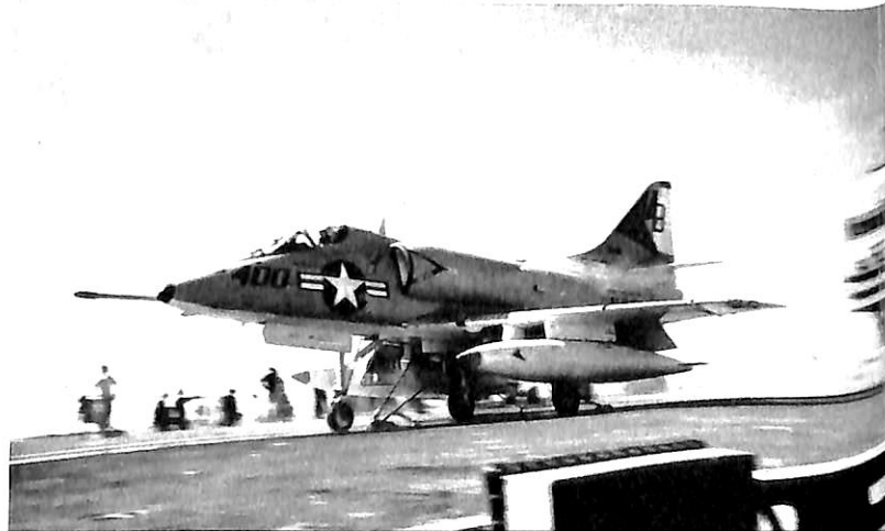
An A-4C Skyhawk attack aircraft gets into motion as it is catapulted from the flight deck.
