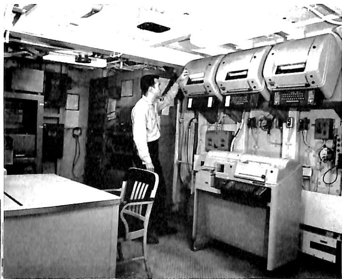
Aerology : Aerographers mate checks incoming weather on a TT/130C teletype
