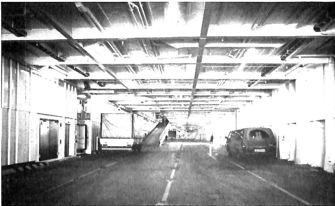
Trailer Deck (8 m Trailer 54, 12m " 19)
