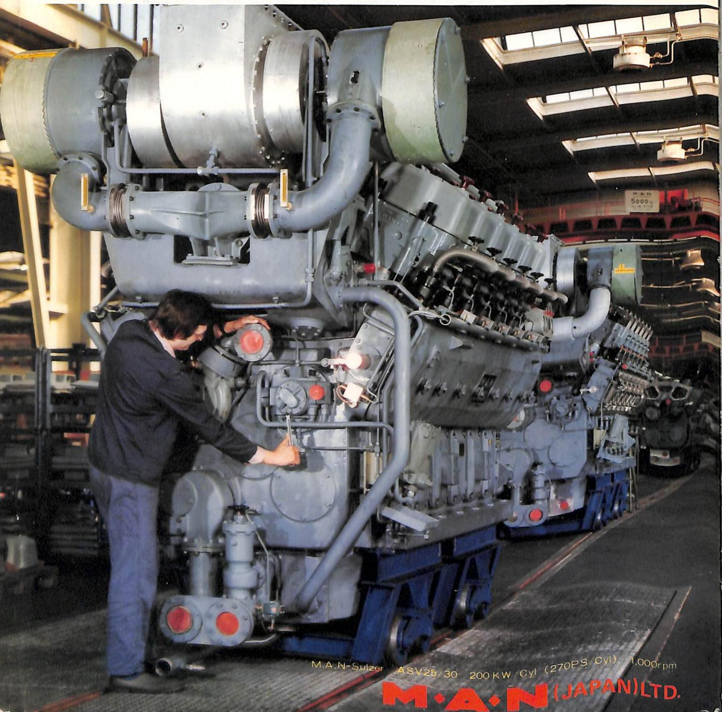
M.A.N-Sulzer ASV25/30 200 KW/Cyl (270PS/Cyl) 1,000 rpm
