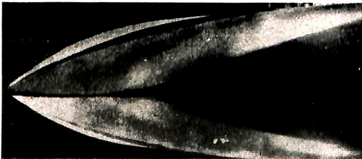
FIG. 4. —LAMINAR FLOW ALONG A 2.5 m HAKUBASAN-MARU MODEL 'WITHOUT' TRIP-WIRE (TOKYO UNIVERSITY TANK, 1951)
