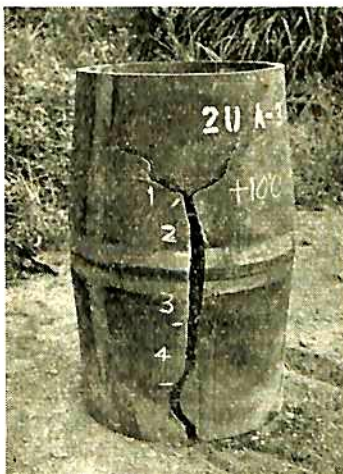
FIG. 17 FRACTURED SPECIMEN OF EXPLOSION TEST ON WELDED TUBE OF QUENCHED AND TEMPERED STEEL 20 MM THICK, SHOWING THAT THE CRACK PROPAGATED ALONG THE AUTOMATIC WELDED JOINT 14)
