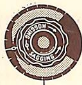
Full width of segment means stresses will be dangerous.
