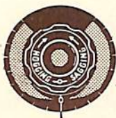
Zero stress reading shows ideal loading condition.
