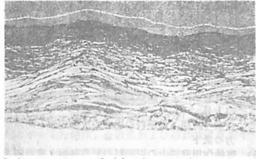
Indicates the scale-like layers of rust being enclosed in FLUID FILM. The particles of rust are softened and finely dispersed and absorbed within the FLUID FILM.
