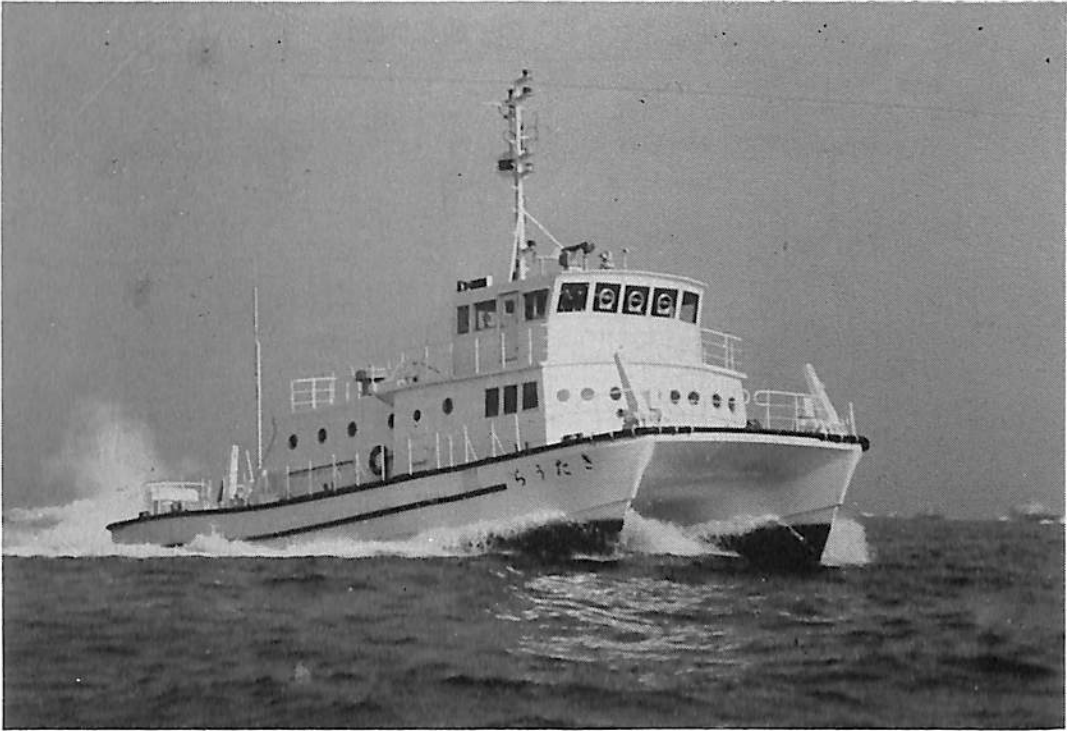
FRP Catamaran Type Surveying Ship "KITAURA" by Technical Division, Japan Aircraft Manufacturing Ltd.
