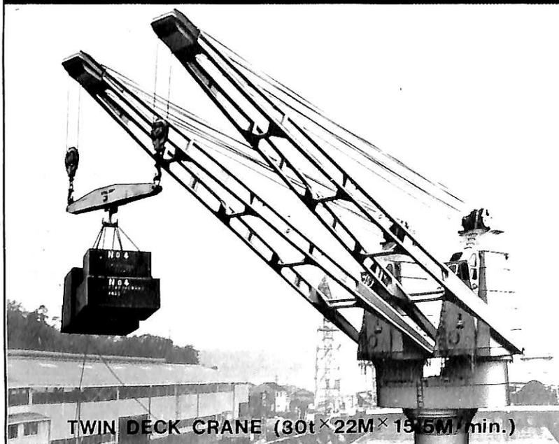
TWIN DECK CRANE (30t×22M×15.5M/min.)
